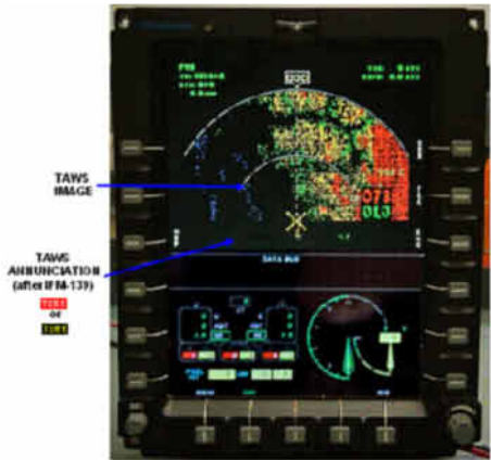
TAWS displayed on MFD Map/Radar page
