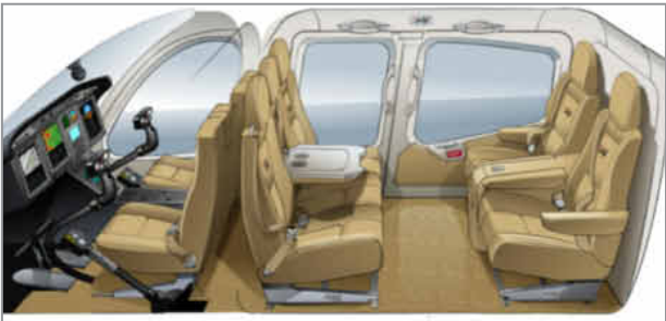
Five place club seating with a row of two 21.5" seats separated by a center console facing a row of three 18.5" seats with a center seat fold-down table.
