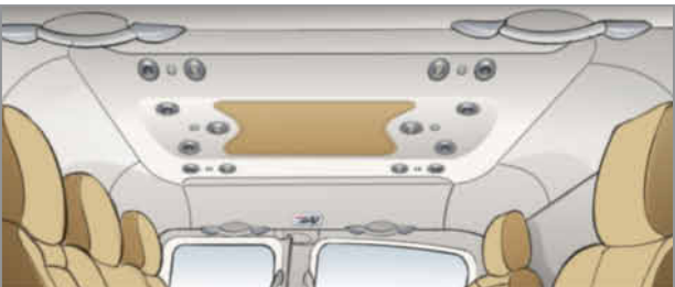
A molded thermoplastic executive headliner with LED lights, adjustable air vents and color coordinated leather trim.
