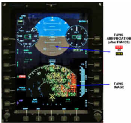
TAWS displayed as HSI underlay on PFD
